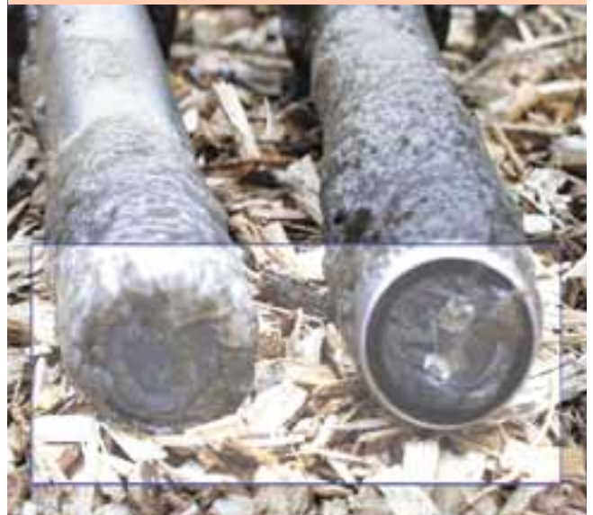
Sensor without and with ultrasound cleaning system after 30 days
